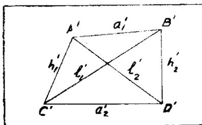
$$\left. \begin{aligned} l_1'^2 &= h_2'^2 + a_2'^2 - 2 h_2' a_2' \cos D' \\ l_1'^2 &= h_1'^2 + a_1'^2 - 2 h_1' a_1' \cos A' \\ l_2'^2 &= h_2'^2 + a_1'^2 - 2 h_2' a_1' \cos B' \\ l_2'^2 &= h_1'^2 + a_2'^2 - 2 h_1' a_2' \cos C' \\ A' + B' + C' + D' &= 2 \pi \end{aligned} \right\}$$
